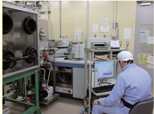
Enrichment Measurement of U using mass spectrometry
